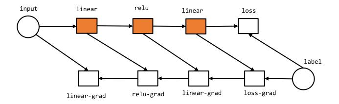
Because the need to keep intermediate value around (checkpoint) for the gradient steps. Training a N-layer neural network would require O(N) memory.
